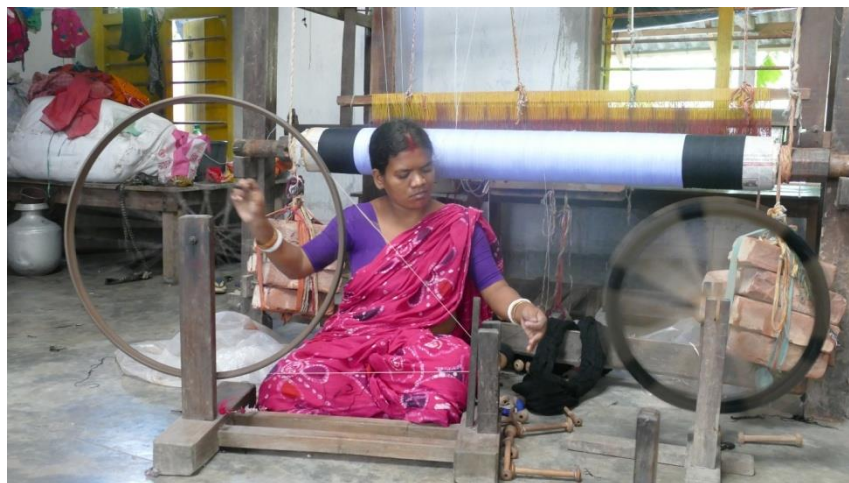
Figure 11: The process of Carding and Spinning of the Jute Fiber
